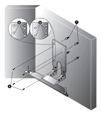
Use (a) holes to attach the VESA mount. Use (b) holes to attach the Wall mount.
